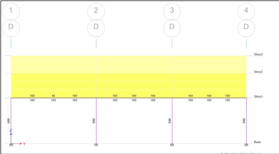
Figure 5-8: Column Design Output Along Grid D-D
